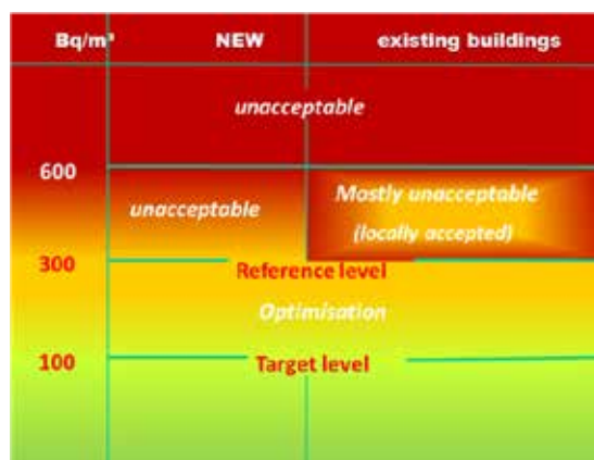
Figure 2. The use of the reference level as a tool for optimisation of the radiation protection.
