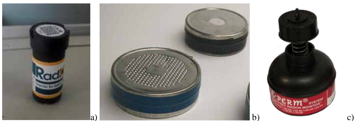
Figure 6. Examples of different types of passive, cumulative radon sensors: a) alpha track; b) activated charcoal; c) electret ionization chamber.
